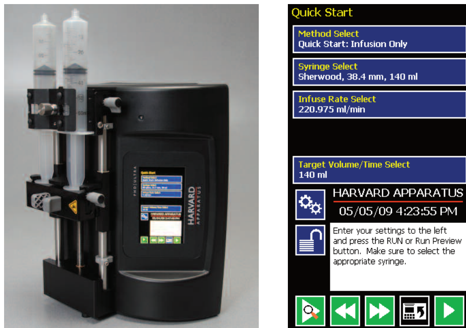
Figure 5: The PHD ULTRA™ pump shown in its vertical (upright) orientation and the associated Quick Start menu screen showing the application auto-rotated into portrait mode.
