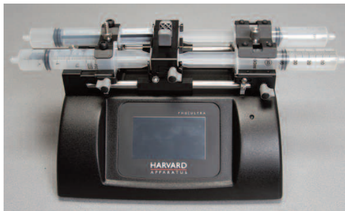
Figure 85: PHD Ultra showing syringes installed on both sides of the Pusher Block.
