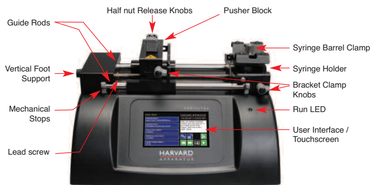
Figure 2: Front view of the PHD ULTRA™ pump with important components and controls.
