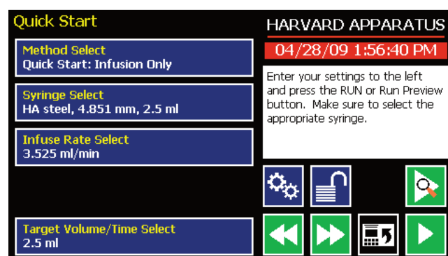
Figure 98: The Time/Date area turns red when the battery is low.
