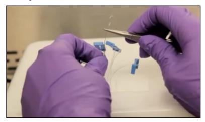
3. Thread the 2<sup>nd</sup> electrode into electrode port 1. Ensure that both electrode tips are touching the glass slide.
