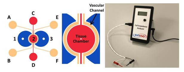
Schematic of the chip used for the SynBBB Model and SynVivo Cell Impedance Analyzer system. Apical chamber (outer channels) are for culture of vascular (endothelial cells) while basolateral chamber (central chamber) are for culture of brain tissue cells (astrocytes, pericytes, neurons). Porous architecture enables communication between the vascular and tissue cells.
